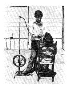
In India and Guatemala, health workers use a foot treadle to power a drill, the same way they operate a sewing machine. This kind of drill is slower than a compressed-air drill, and the grinding produces a lot of heat, so one must take care not to let the tooth get so hot that it kills the nerves (see p. 146). Still, this is one of the simplest and cheapest ways to place a permanent filling.
