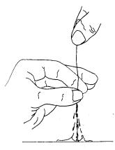
(1) Soak thin string in hot wax. (2) To remove the extra wax, pull the string between your fingers.
