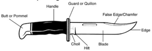
Every knife needs sharpening from time to time. With the following instructions, you will be using the safest and most effective method of sharpening your knife. Never sharpen your knife on a power-driven grinding wheel. This can burn the temper from your blade, which will make the edge brittle and possibly chip or crack.
