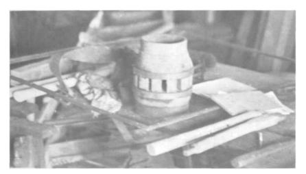
PLATE 79 John used a factory-turned hub for our wheel—ready for use except for the addition of the four bands. Traditionally the hubs would be turned on a foot-powered lathe, and the slots for the spokes cut with a sharp chisel. Here, the hub is ready for the last band to be added.
