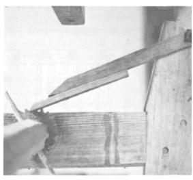
**PLATE** 289 Brace (clutch) mounted to side (inside) of frame to articulate with cogs and hold cloth beam steady and in place so threads are kept taut.
