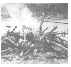
PLATE 146 With the four buckets that cut across the grain roughed out, Sam now takes two iron wagon wheel rims, each thirty-six inches in diameter, builds a fire around them (one can use hickory, corn cobs, or any-thing else that burns evenly and well), and gets them red-hot.
