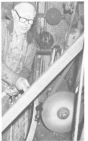
PLATE 110 Now he gets the tire red-hot in his forge. He moves the tire about a foot at a time through the flames until it has gone about four complete, very slow revolutions.
