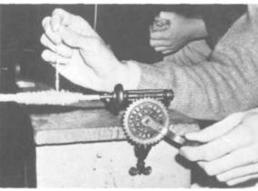
PLATE 250 When the warp is in place, the weaver loads the bobbins for the shuttles. Often a BOBBIN WINDER is used for this, as seen here. Bobbins can be loaded either directly from a skein mounted on a swiss, or from undyed thread still on broaches.
