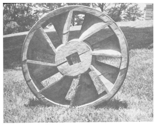
PLATE 153 The finished wheel from the bottom side.
