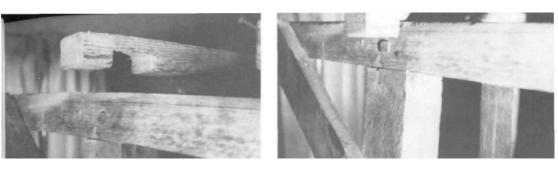
PLATES 261-262 These two photographs show how the frame that holds the heddles (the fifty-two-inch bar) fits down over the top of the loom frame. It is not held in place by anything other than notches.
