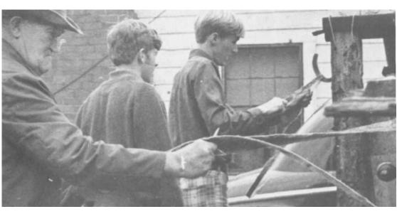
PLATE 170 The frame finished, the foot pedal is now mounted to it. Choose two four-foot 2X4S. Here Minyard sharpens one end of each so they can be driven into the ground. (Note: As in *Plate 171*, they are driven into the ground on a slant, about shoulder width, or 3/2 feet, apart.)
