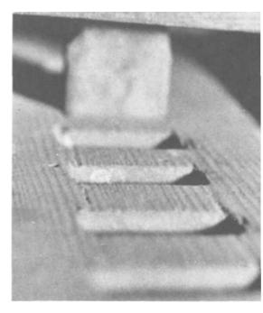
PLATE 287 Detail showing slots cut in top of loom frame to hold the beater frame.
