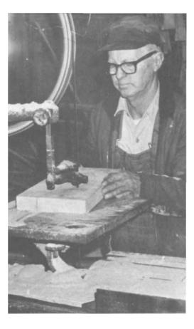
PLATE 95 He drills the holes for the ends of the spokes with a drill press, rather than with the auger which would have been used traditionally. He drills the holes from the inside of the felloe.
