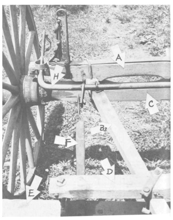
PLATE 120 Brake assembly. See diagram in Plate 121.
