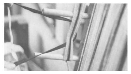
PLATE 292 Mrs. Brown ties a ribbon around the cross made by the warp threads between pegs 1 and 2. This step is necessary to prevent the threads from getting mixed up and out of order when they are taken off the frame. (Note the different colors of threads in place in the same position they will hold when the warp is put on the loom.)
