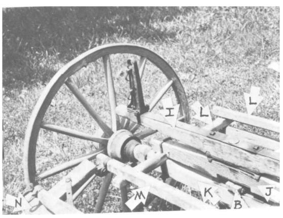
PLATE 122 The front axle assembly. See diagram in Plate 123.
