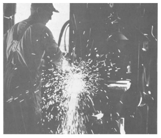
PLATES 81—82 Now the rough edges left by the weld are ground off. The band is next heated red-hot in the forge, driven onto the moistened hub, and then doused with water to make it contract and hold.
