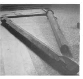
PLATE 274 Breast beam from bottom with cloth beam in back-ground.
