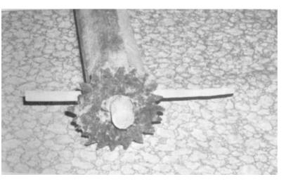
PLATE 283 Opposite end of beam showing metal cog.
