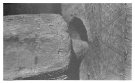
PLATE 282 This end of •loth beam is hewn into a knob to fit into hole in loom frame.
