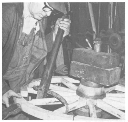
PLATE 103 When the felloes are in place, John takes a hand saw and saws down between each seam to insure that they meet flush, and are lined up correctly.
