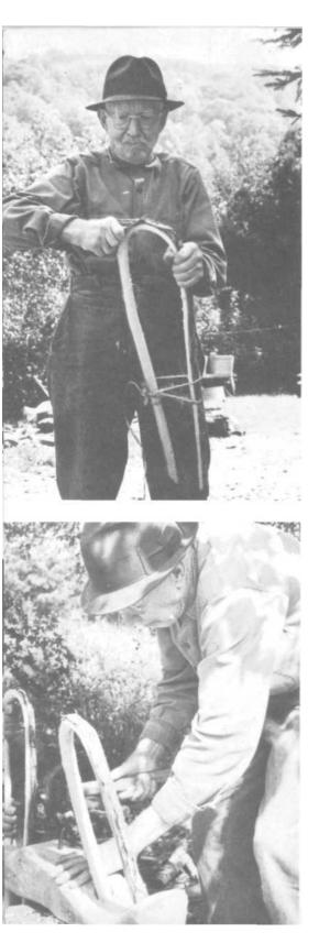
PLATE 71 The bow could be left tied if desired, and set up in the barn loft to season and "set." For our purposes, however, that wasn't necessary. Mr. Barnes simply went ahead and trimmed off any splinters . . .
