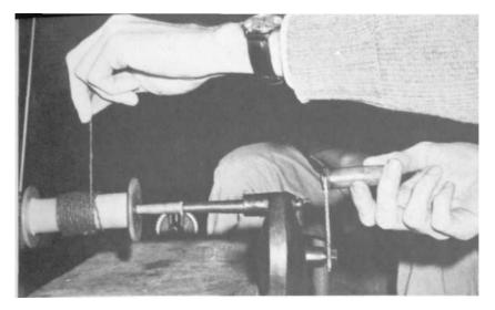
PLATE 246 Now a spool is mounted on the SPOOLER directly below the swiss, and thread from the skein fed onto the spool. As the spooler's crank is turned, the swiss turns also, feeding thread into the spool until it is full, at which point it is replaced by another. Spools can also be filled from broaches (filled bobbins off the spinning wheel) if desired. The swiss would not be used in this case, however.
