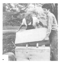
PLATE 132 The slab with the pegs in place is now lifted onto its mate, pegs and holes are matched . . .
