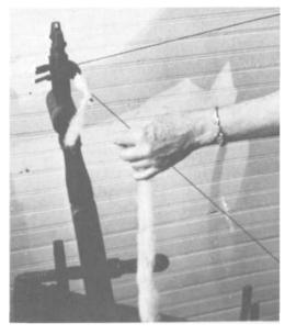
PLATES 214-215 Dean Beasley shows us how to spin using one of Margarets rolls. Her corn shuck bobbin (Plate 198) was already in place on the spindle as she had been spinning (Plate 214). She simply look the end of one roll and pressed it against the tag end of the roll she had been spinning (Plate 215), and
