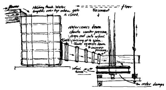
PLATES 158-159 This diagram shows the holding tank and chute assembly in the Watts mill. The chute is also shown in *Plate 159*.
