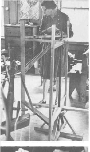
PLATE 249 Dean uses a WARPER like the one shown here rather than use the more traditional warper described later. One revolution of the warper (bottom peg to top peg) equals three yards. When Dean weaves a three-yard piece the width of a stole (230 threads), she mounts ten spools in the spool rack, and goes from top pegs to bottom pegs twenty-three times. As each spool runs out, she mounts a full spool in its place, ties the thread ends together, and continues.
