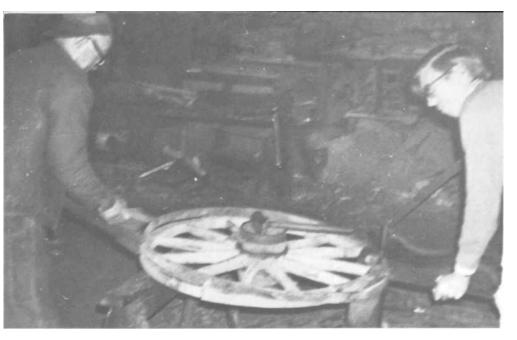
PLATES 111—113 Moving quickly, he carries the tire to the wheel, has a second person clamp down on the opposite side to keep the tire from flipping up (*Plate HI*), and pulls the tire over the rim of the wheel with a "tire puller" (*Plates 112-113*).
