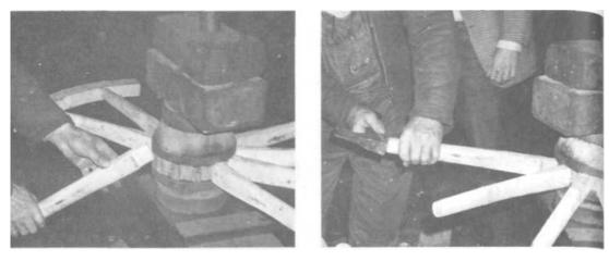
PLATES 96-97 Next the spokes are driven into the mortises in the hub. No nails or glue are needed. The slope of the mortises in the hub automatically creates the required "dish."
