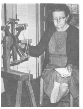
PLATE 242 When Dean has the bobbins completed and ready to be dyed, she winds them off, one at a time, into skeins. Each full bobbin makes one skein.
