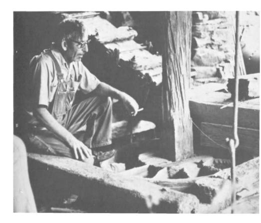
PLATE 160 Sharpening millstones as they get worn through use is one of the trickiest jobs involved in running a mill. The fans are recut periodically by slowly and painstakingly pecking away at them with a hammer like the one Sam is using. Sam never "beats" on the rock—he just taps lightly hour after hour until the sloped surfaces of the fans are just right.
