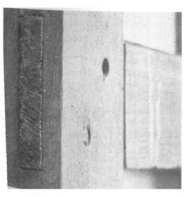
**PLATE** 288 Detail showing how side **beam** fits **into loom leg. Note** mortise <sup>in</sup>i(| tenon **joint** wilh **pees.**
