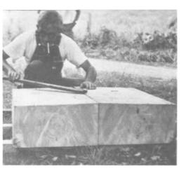
PLATE 134 Sam now finds dead center of the top surface. He drives a nail through a stick of scrap wood into dead center, measures out eighteen inches from dead center on the stick, and drives a second nail through this point. With the point of the second nail, he scribes a circle thirty-six inches in diameter on the top surface.
