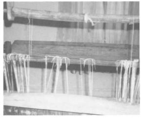
PLATE 265 One heddle in place on a harness. Thread (warp thread) passes through the central eye.
