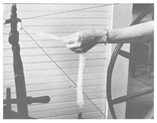
PLATE 216 ... holding the ends together, she slowly turns the wheel and draws back gently with her left hand, being sure to keep the thread spinning on the very tip of the spindle by  $\ldots$
