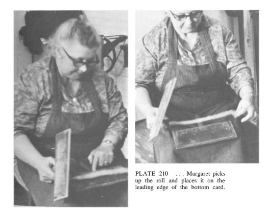
' LATE 209 Then, using several strokes of motion E, she gently nudges the roll backwards. This helps to gather the fibers and consolidate the wool into an actual «oll." When the roll is at the back of the bottom card
