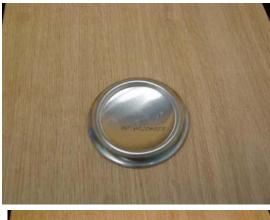
This is a picture of a "raw" aluminum can bottom. I cut the bottom off just to make storage of the reflector a bit easier.
