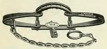
Spread of Jaws, 6½ inches. This trap is the same in size as the No. 4 Beaver, but has heavier and stiffer springs and offset jaws, which allow the springs to raise higher when the animal's leg is in the trap, and is furnished with teeth sufficlently close to prevent the animal from pulling its foot out.
