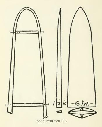
small wire nail at each end. A handful of shingle or lath nails and a clump of osier sprouts will make a full outfit of stretchers for a temporary camp.
