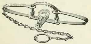
Spread of Jaws  $4\frac{7}{8}$  inches. The No. 2 Trap is called the Fox Trap. Its spread of jaws is the same as the No.  $1\frac{1}{2}$  but having two springs it is, of course, much stronger.
