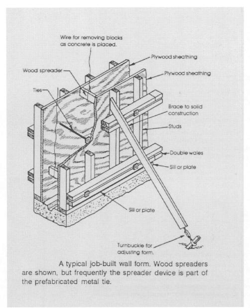
After the concrete has set, the clamps can be quickly removed and the forms stripped. A special wrench is used to break off the outer sections of the rod. The rod breaks at a small indentation located about 1 in. below the concrete surface. The hole in the concrete is patched with grout or mortar, completely embedding the remaining portion of the tie and providing a smooth surface.
