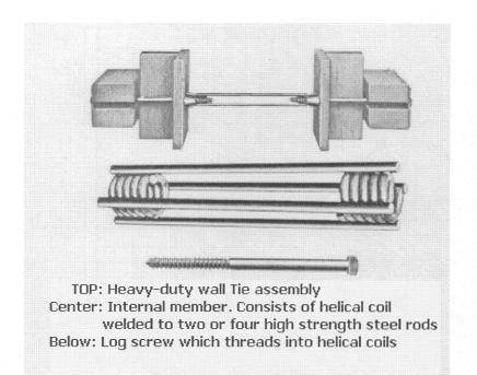
Other types of patented wall ties are shown in the above figure. The coil type spreader is assembled with a cone of wood, plastic or metal
