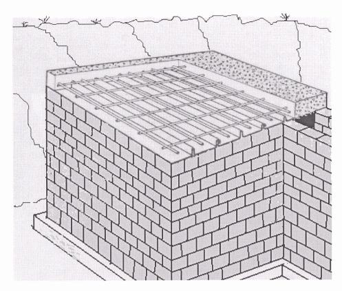
A band will be constructed around the outside perimeter of the foundation using 2x10 or 2x12 scrap lumber. The slab thickness will be 6" however the overlay will be fastened to the completed foundation wall to hold in the concrete in the liquid state. Make sure that you brace the band with 2x4's securely staked to the ground.
