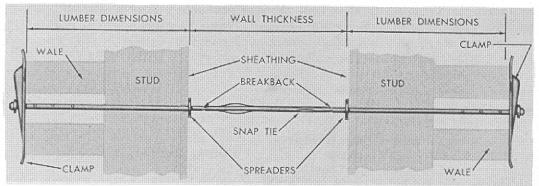
The Figure above shows a type called a snap tie. This is available for various wall thickness. The rod goes through small holes bored through the sheathing and studs. Holes through the wales can be larger for easy assembly or the wales can be doubled as shown. The spreader washer is rigidly set on the tie rod, thus holding the forms apart.
