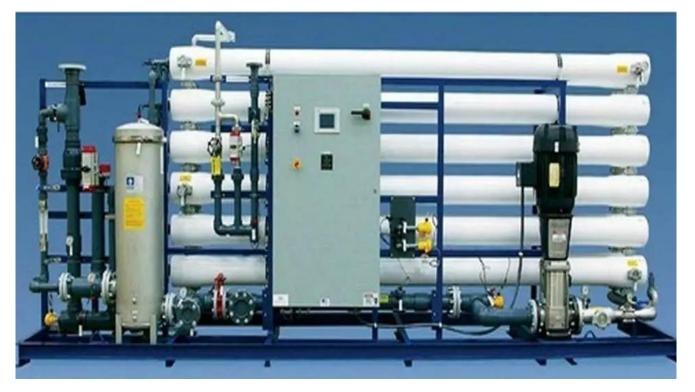
Nanofiltration hasn't quite taken off yet but is still an incredibly viable way to get purified water. Much like reverse osmosis, <u>nano filter membranes</u> are semi-permeable. Unlike reverse osmosis, they are more permeable which allows more water to be processed at once.
