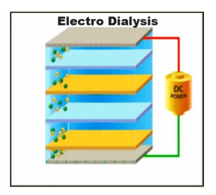
Probably the most complicated method on the list and only used by commercial projects, <u>EDR</u> uses the power of electricity to purify seawater for consumption.
